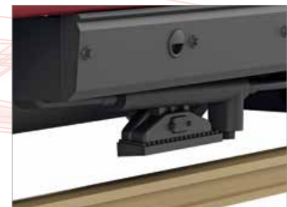
■ Train control magnet
