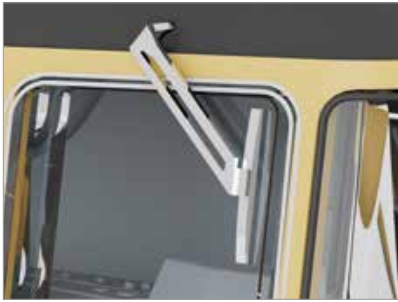
■ Separately attached windscreen wipers
