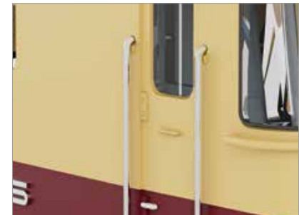
■ Handle rails on the access points made of metal
